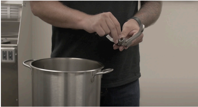
2. Place key way back into replacement blade.
