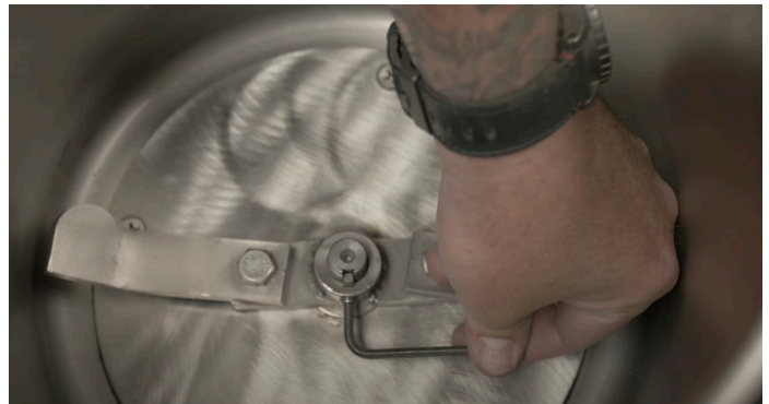
7. Replace set-screw and tighten with allen wrench.
