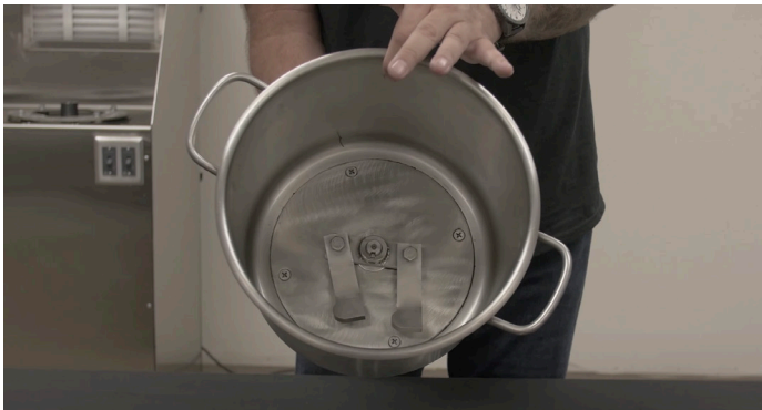
6. Make sure blade lays on top of washer welded to bucket.
